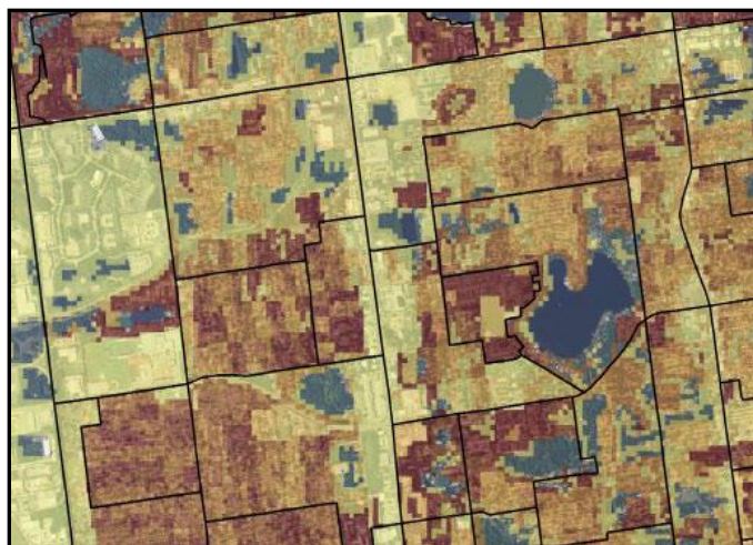
A dasymetric population map for several census blocks in Tampa Bay, FL. A single census block may have pixels that are non-habitable, as indicated in blue, as well as a range of low, medium, and high-density land cover types indicated in shades of red—the darker the pixel, the greater the population density.
