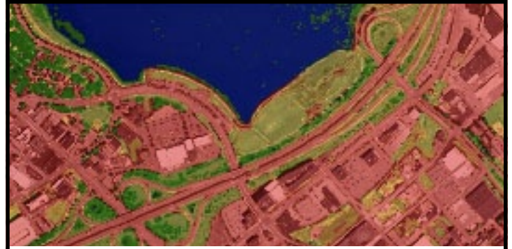
Aerial photography of downtown Portland, ME, classified into vegetation (greens), impervious surfaces (pink), and water (blue)
